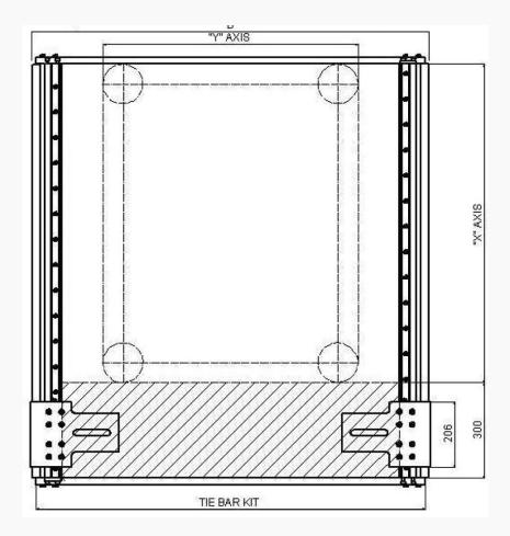
Gantry base is used to maximize our 2 Axis Milling Beam potential and enable accurate milling over a large 3 Axis area to be used insitu. A perfect machine for levelling Engine mounts, pump and motor pads, heat exchangers division slots and plates, split lines, press beds and many more
